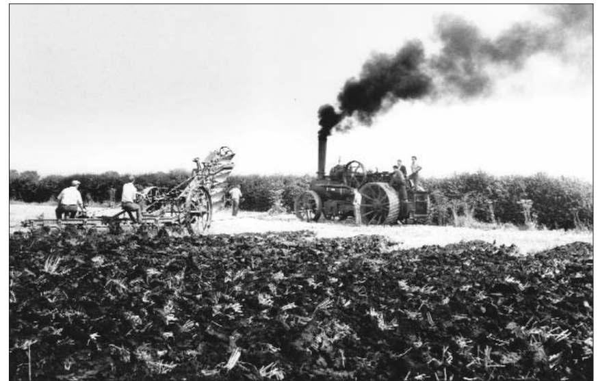
Fowler ploughing engine and a 7-furrow balance plough at work in a ploughing demonstration at Roxton Park, Bedfordshire in 1986 (photograph: John F. Clay)
