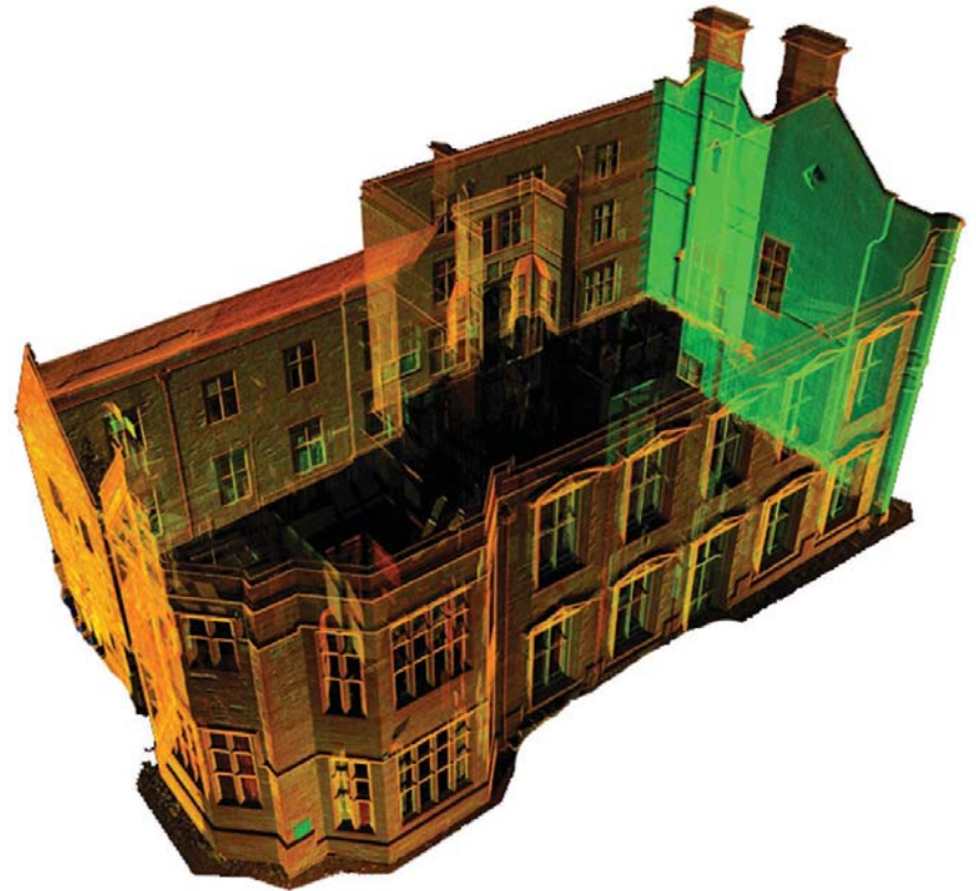
Laser scan of Staveley Hall, Derbyshire (reproduced by permission of Marcus Abbot; © ArcHeritage)
