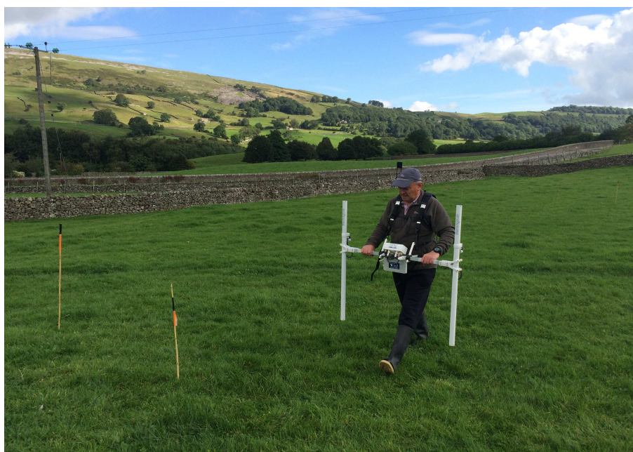
Plate 2: One of the SWAAG members undertaking magnetic survey.
