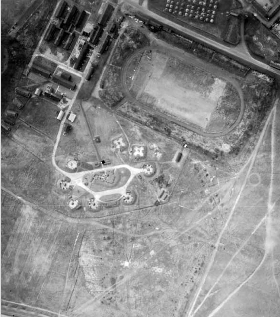
Figure 13: The Second World War Heavy Anti-Aircraft Artillery battery on Woolwich Common in October 1945 (North is to the right of the photograph). The original octagonal, and two variations of later square, gun emplacements are visible as well as the hutted camp that supported the battery to the south-west (top-left) and the sub-circular mark left by the gun laying radar mat to the bottom (east). The oval outline of Woolwich stadium is also clearly visible at the top (west) of the photograph. (RAF 106G/UK/916 6087 11-OCT-1945) English Heritage (NMR) RAF Photography.
