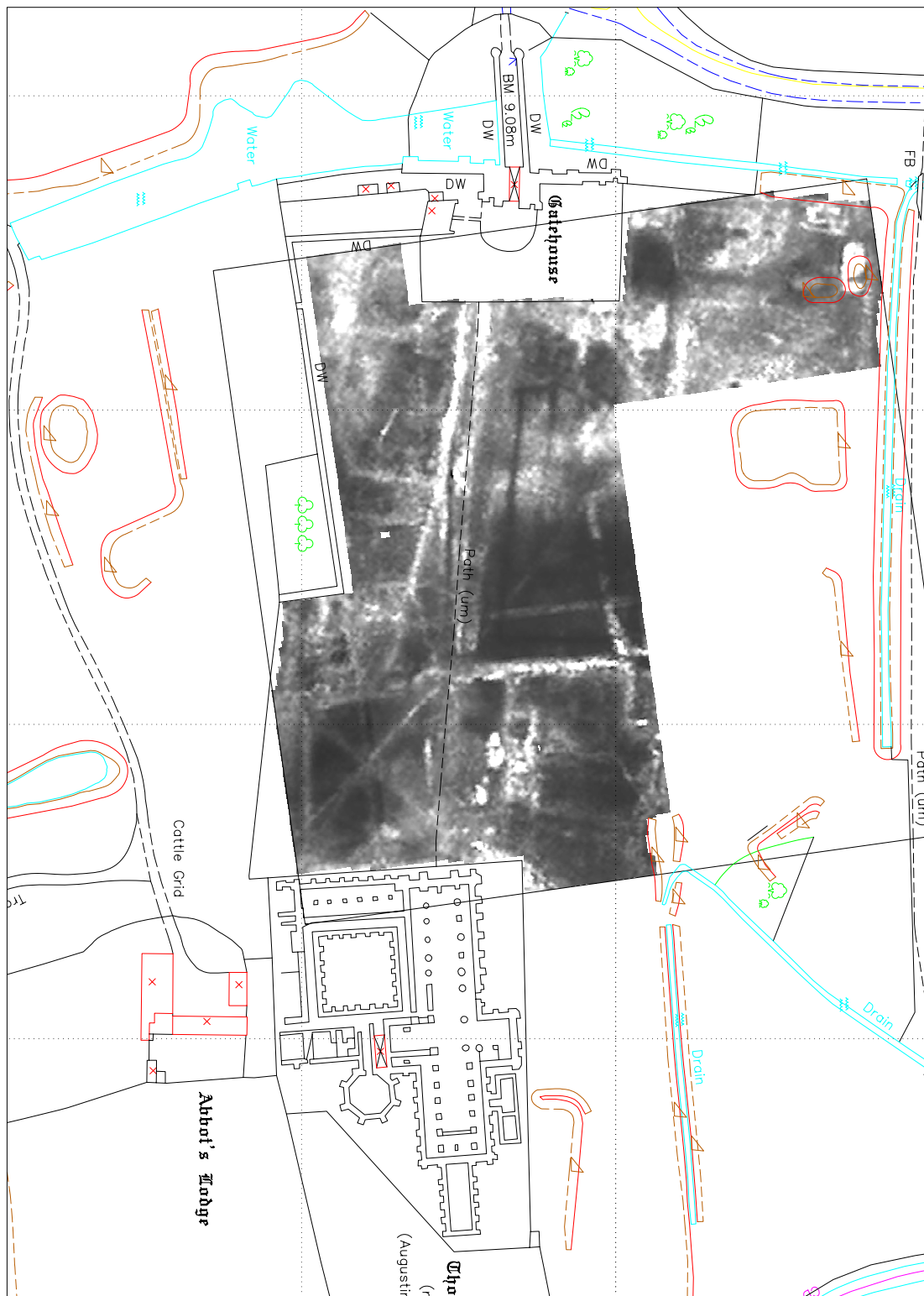
Figure 27. Earth resistance survey data, reduced from original plot at 1:1,250 scale.
