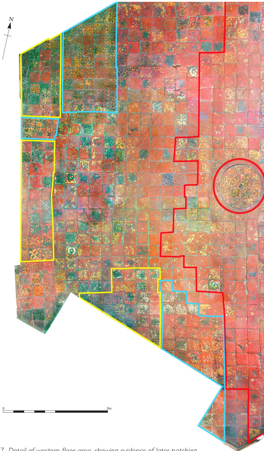
Figure 7 Detail of western floor area, showing evidence of later patching.
