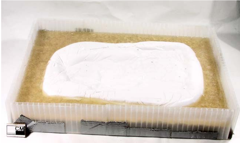
Fig 30 : Correx box former, with curing epoxy/Vermiculite mix surrounding the silicone rubber inner mould
