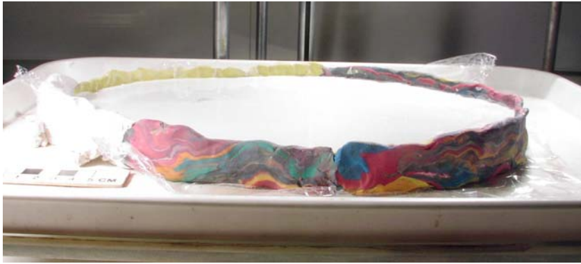
Fig 29 : Construction of the cushioned mould, with silicone rubber curing inside a plasticine dam
