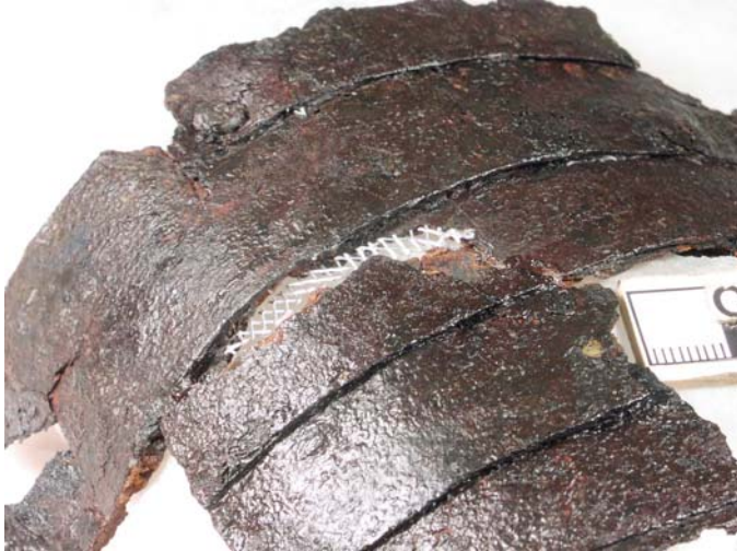
Fig 17 : Aluminium mesh tacked in place with Paraloid B72
