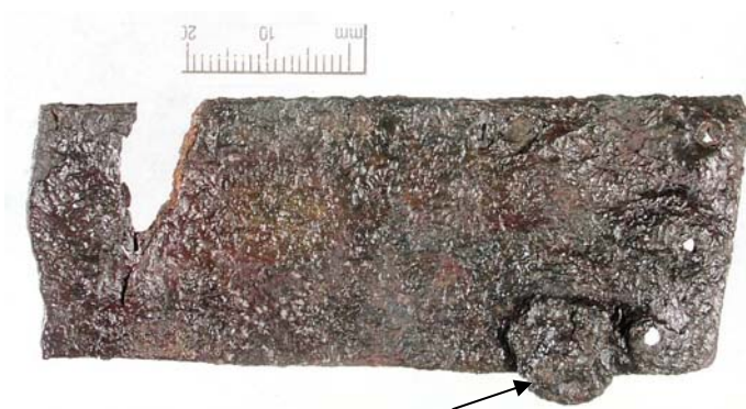
Fig 15 : 3979BΔ/9 showing iron rivet
