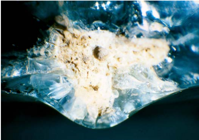
Fig 4 : Possible nodule of slag in the vessel wall (X16)
