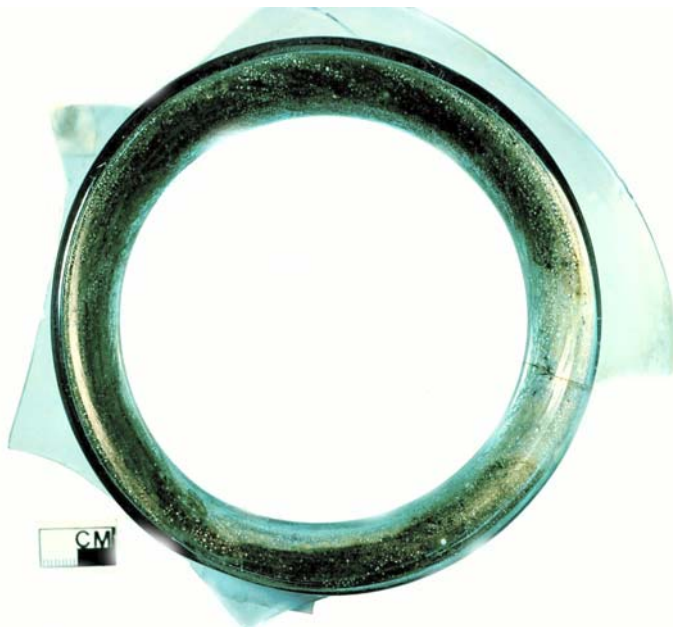
Fig 1 : Discolouration of the rim caused by biological slime
