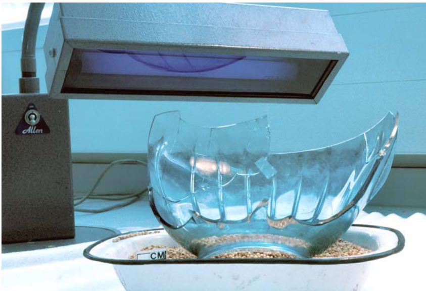
Fig 2 : Cyanoacrylate adhesive curing under UV light
