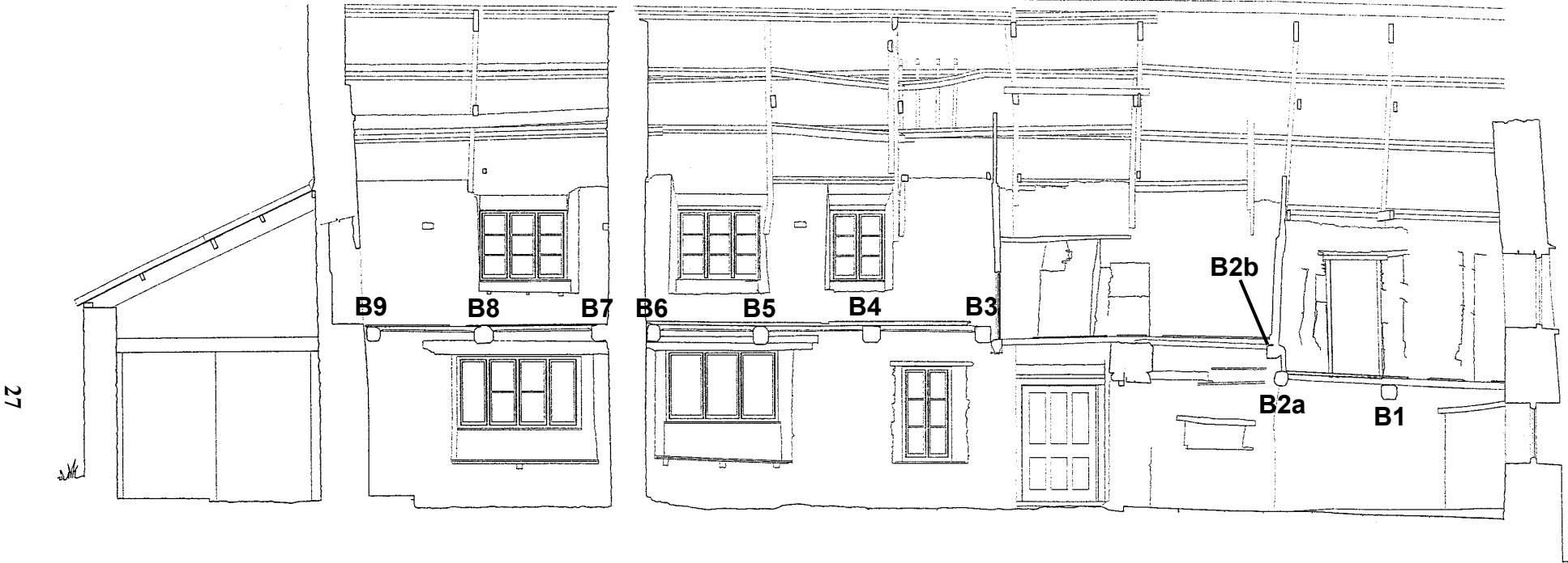
Figure 15 Section through the north range, north face of the south wall, showing the ceiling beam numbering scheme including B2a and B2b (after English Heritage drawing AS8/004 by Selwood 1995)
