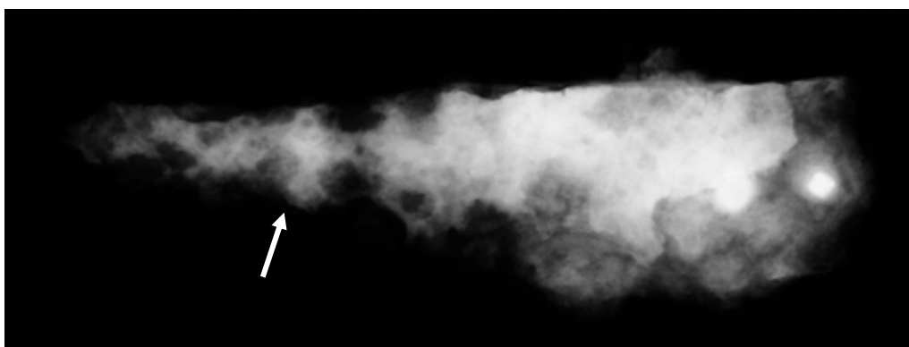
Figure 2. X-radiograph showing the blade to the left and the riveted plate-tang of the handle to the right. The arrow marks the position from where the metallographic sample was removed.
