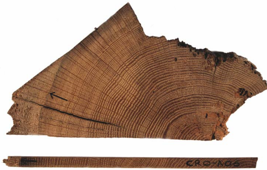
Figure 2: Cross-section of a rafter showing the presence of sapwood rings in the left hand corner, the arrow is pointing to the heartwood/sapwood boundary (H/S). Also a core with sapwood; again the arrow is pointing to the H/S. The core is about the size of a pencil.
