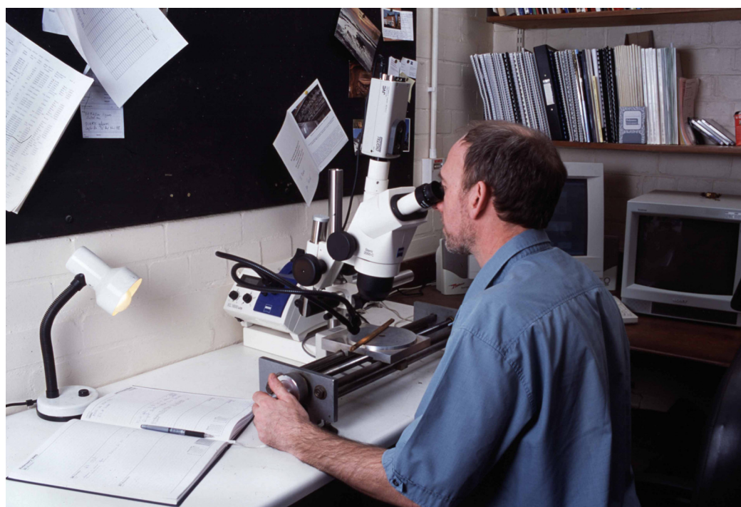
Figure 3: Measuring ring widths under a microscope. The microscope is fixed while the sample is on a moving platform. The total sequence of widths is measure twice to ensure that an error has not been made. This type of apparatus is needed to process a large number of samples on a regular basis.
