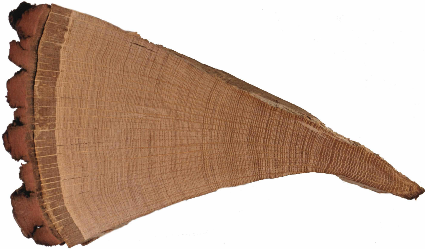
Figure 1: A wedge of oak from a tree felled in 1976. It shows the annual growth rings, one for each year from the innermost ring to the last ring on the outside just inside the bark. The year of each ring can be determined by counting back from the outside ring, which grew in 1976.
