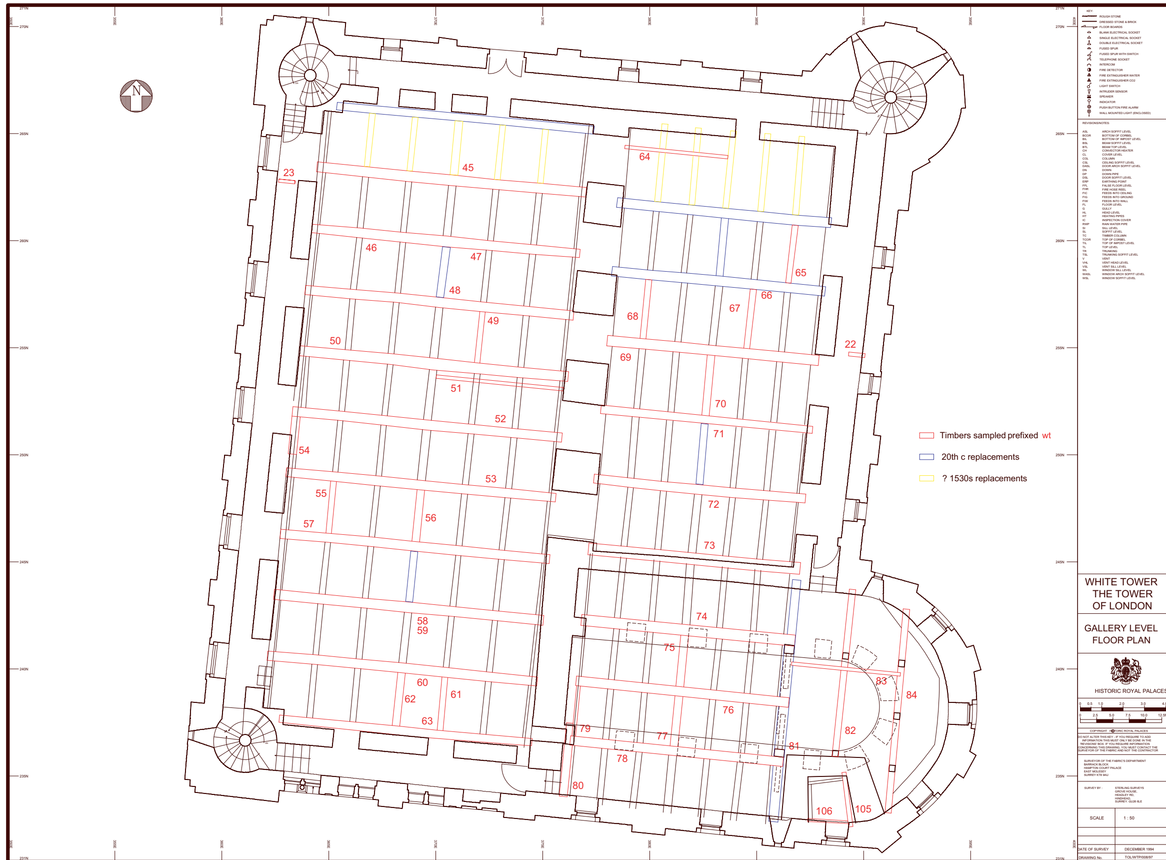
Figure 49: Plan of second-floor level showing locations of timbers sampled (after Historic Royal Palaces)
