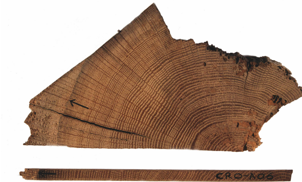
Figure 2: Cross-section of a rafter showing the presence of sapwood rings in the left hand corner, the arrow is pointing to the heartwood/sapwood boundary (H/S). Also a core with sapwood; again the arrow is pointing to the H/S. The core is about the size of a pencil.
