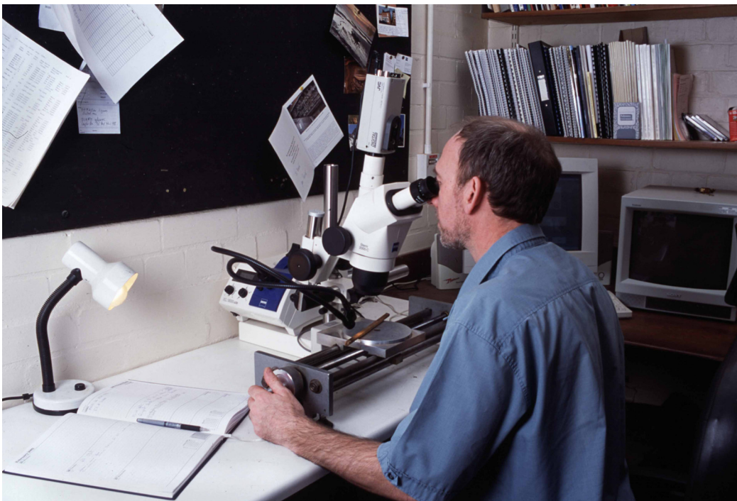
Figure 3: Measuring ring widths under a microscope. The microscope is fixed while the sample is on a moving platform. The total sequence of widths is measured twice to ensure that an error has not been made. This type of apparatus is needed to process a large number of samples on a regular basis.
