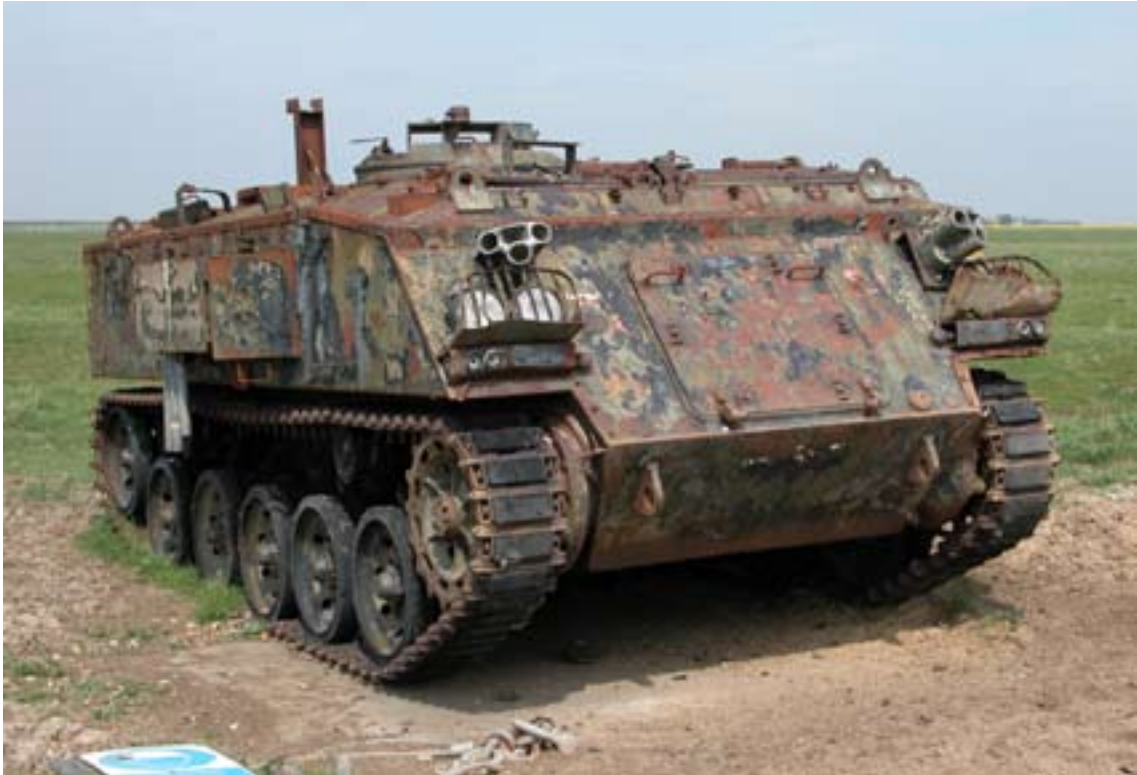
Figure 33: FV432 armoured personnel carrier that was used as a mobile protected shelter. (c) English Heritage
