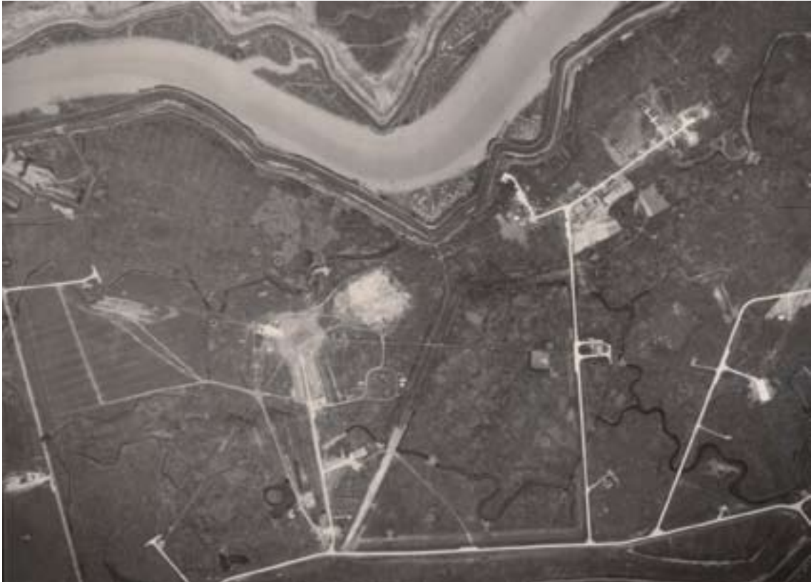
Figure 11: Range I, or the Large Bomb Range, later split into ranges C, D, F and I. In the centre two large scars may be seen formed by detonating large amounts of high explosives, faint linear lines from these areas mark the position of command and instrumentation cables. (c) Crown copyright NMR RAF (V) 542/201 0012 30 June 1955
