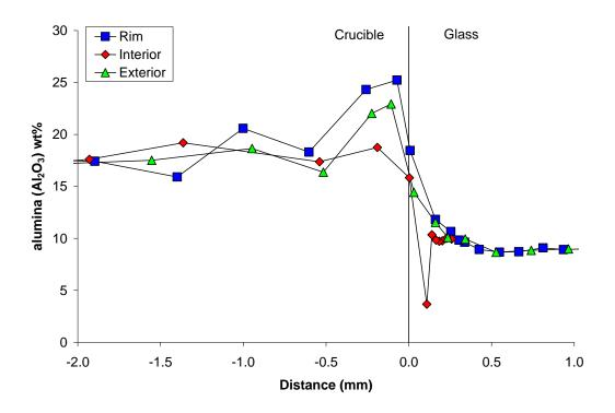
Figure 6. Linescan showing changes in aluminium concentration through the ceramic fabric and surface vitrification/adhering glass of crucible 3
