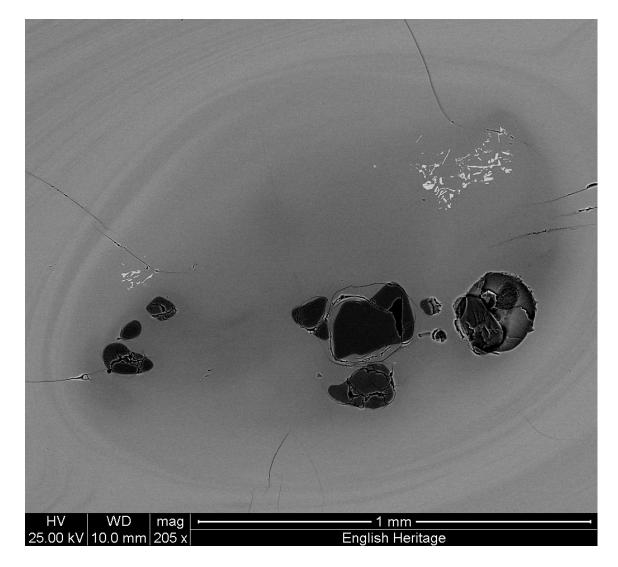
Figure 4. SEM image of sample 5 (back-scattered electron detector, brightness is proportional to average atomic number). The rounded dark patches in the centre of the images are silica while the small bright areas near the top right are crystals of wollastonite
