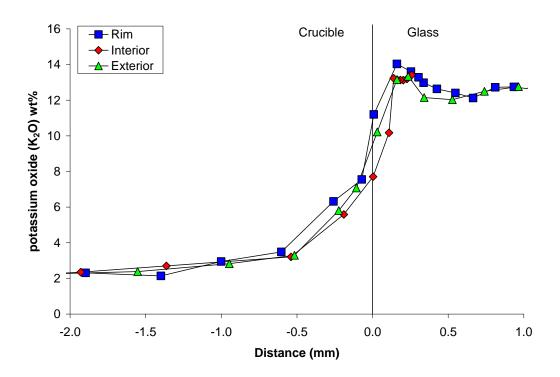
Figure 7. Linescan showing changes in potassium concentration through the ceramic fabric and surface vitrification/adhering glass of crucible 3
