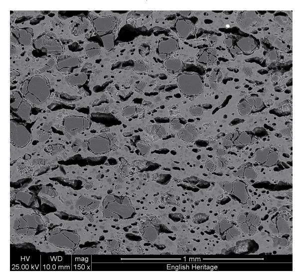
Figure 5. SEM image of sample 3 (back-scattered electron detector, brightness is proportional to average atomic number). The black areas are porosity, the dark grey areas are silica and the remaining light grey areas are the vitrified ceramic
