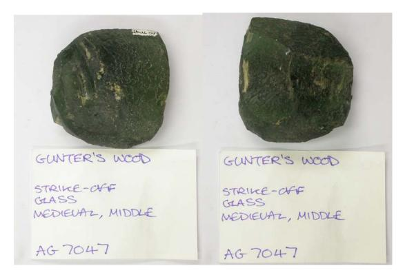
Figure 2. Exterior (left) and interior (right) views of the moil fragment (sample 2).
