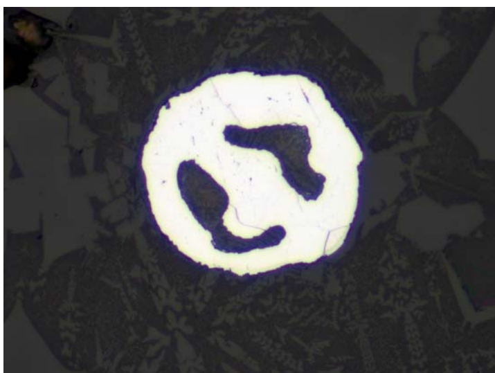
Fig 47. Optical micrograph of a spherical prill with ferrite microstructure in LF02.
