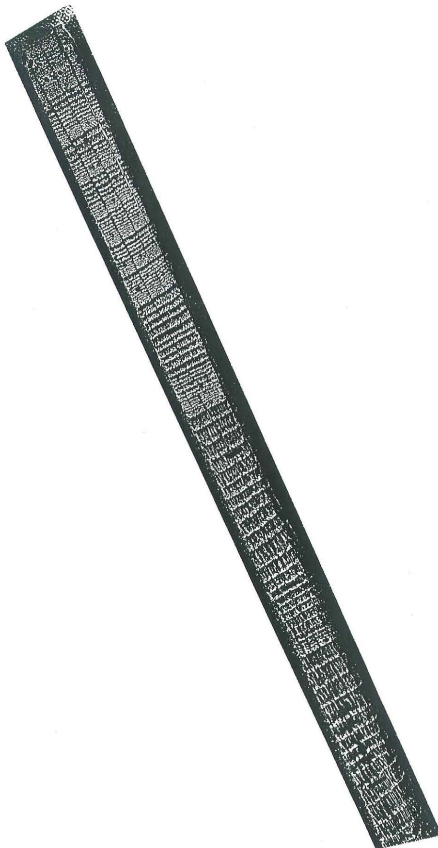
Figure 5: Illustration of erratic growth-ring pattern in undated sample HED-B01
