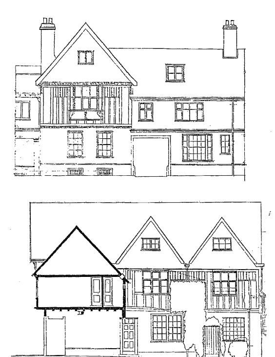
Figure 4: Front (upper) and side (lower) elevations of Nos 80 and 80A Fore Street, Ipswich
