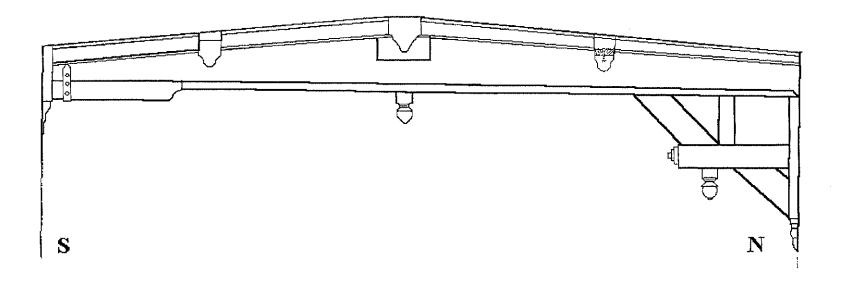
**Figure 1:** Cross-section of the central trusses of the roof of the Chicheley Chapel, St Andrew's Church, Wimpole, Cambridgeshire, showing the form of the false hammerbeam remaining on the north side and its replacement by a single support on the south side.
