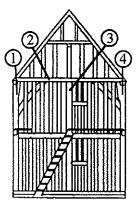
d. View D: Central truss of east wing, showing location of sampled timbers 5 and 6 (after Bond pers comm)
