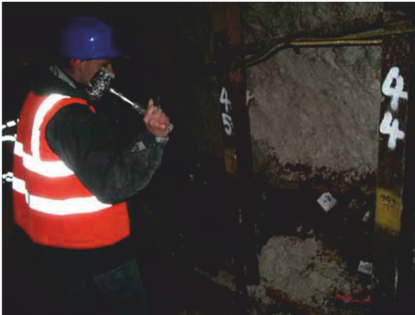
Figure 1: Sampling under subdued red-lighting conditions; photograph was taken using flash photography. The light-exposed outer portion of each sample was removed prior to taking the sample from the section (Photo: H M Roberts)
