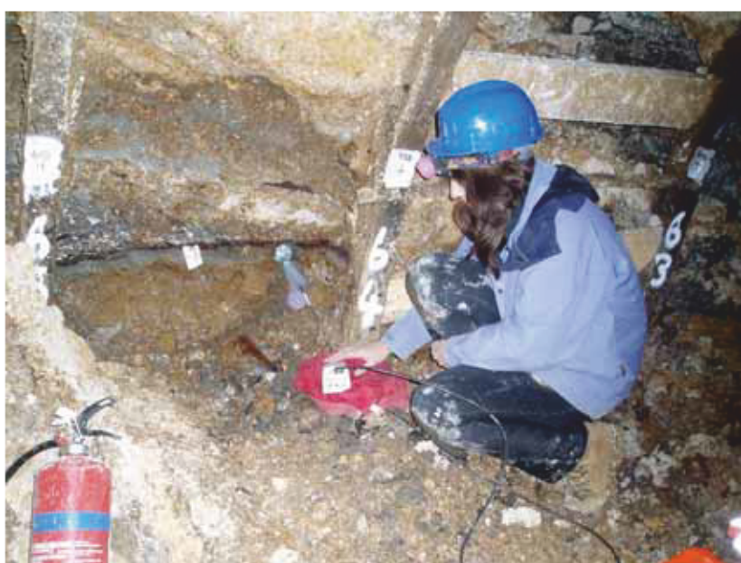
Figure 2: Taking in situ field gamma spectrometry measurements (Photo: G A T. Duller)
