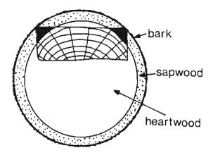
Fig 1: Drawing showing the section of tree trunk used for the Aydon Castle timbers.
