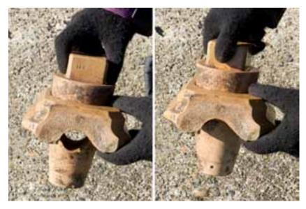
Figure 45: Part of an earthenware acid valve found near acetone recovery house **132**, shown open (left) and then twisted 90 degrees to closed (right). NMR DP141559 and DP141560 07-Mar-2011, Steve Cole © English Heritage.
