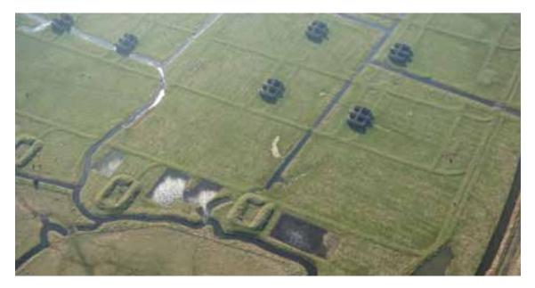
Figure 31: Embanked tramway earthworks clearly visible running between buildings in the north-east corner of **Area K**, looking south-west. Also note the blocks of marsh drainage ridges underlying the factory features, and the unusual instance of paired parallel tramways (right hand side). Extract from NMR 26892/030 08-Mar-2011, Damian Grady © English Heritage.
