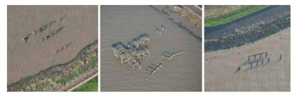
Figure 43: (left to right) Remains of wooden jetty structures **J2**, **J3** and **J4**; note how they are all now cut off from the shoreline. Extracts from (left to right) NMR 26892/028, 26891/044, and 2682/032 08-Mar-2011, Damian Grady © English Heritage.
