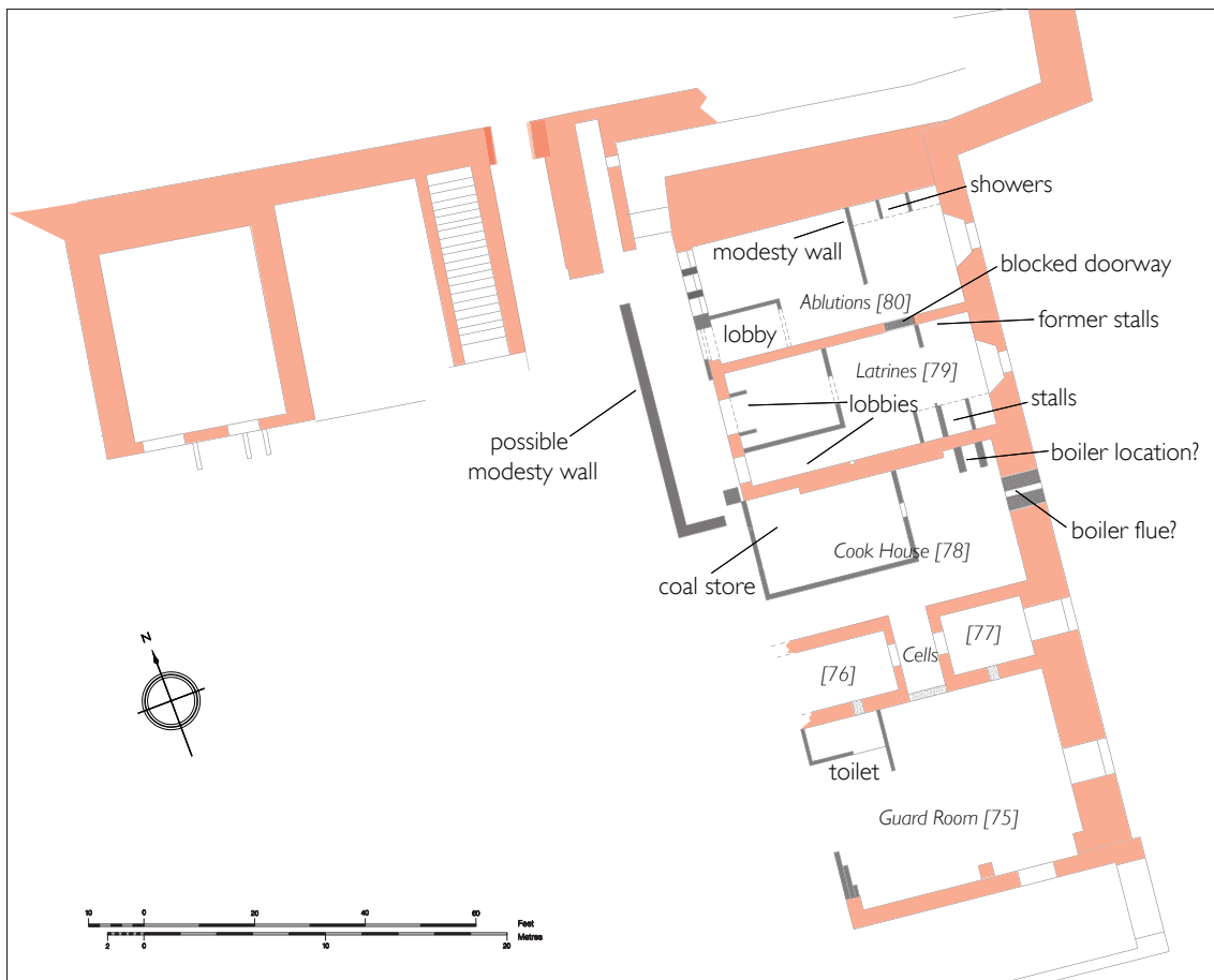
Figure 81: Sketch survey of the rebuilt northern end of the entrance range based on field measurements and the 1899 basement plan (TNA: WO78/4963). The possible Second World War additions and alterations are shown in light grey.
