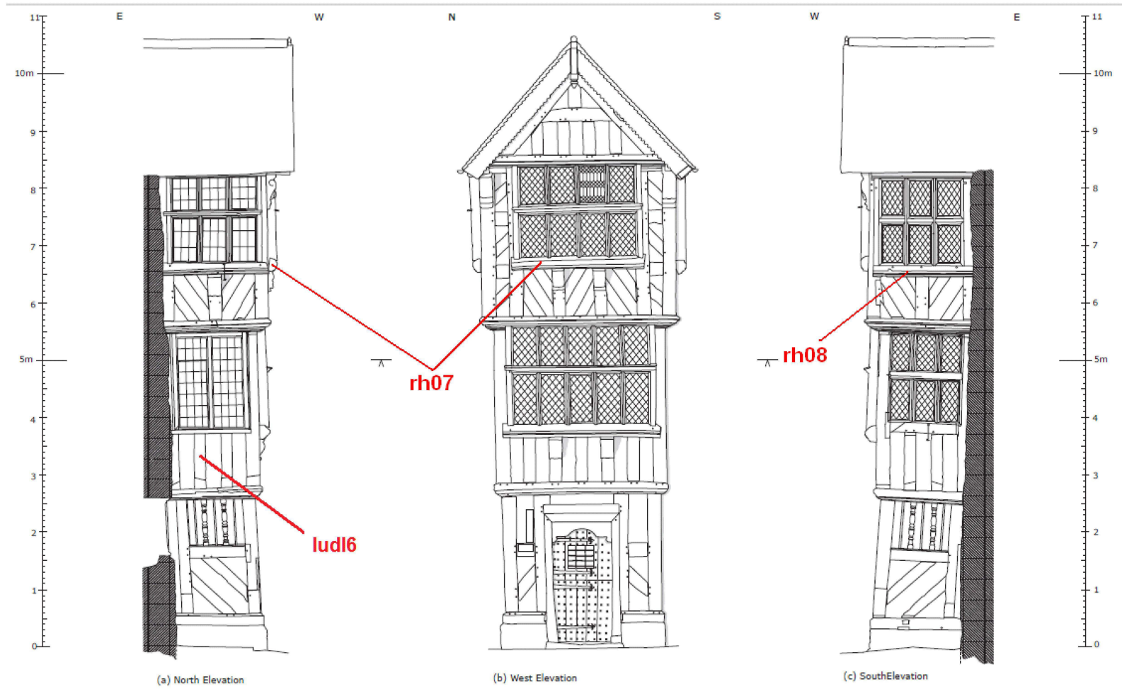
Figure 11: The porch, showing timbers sampled for dendrochronology (after Tyler)
