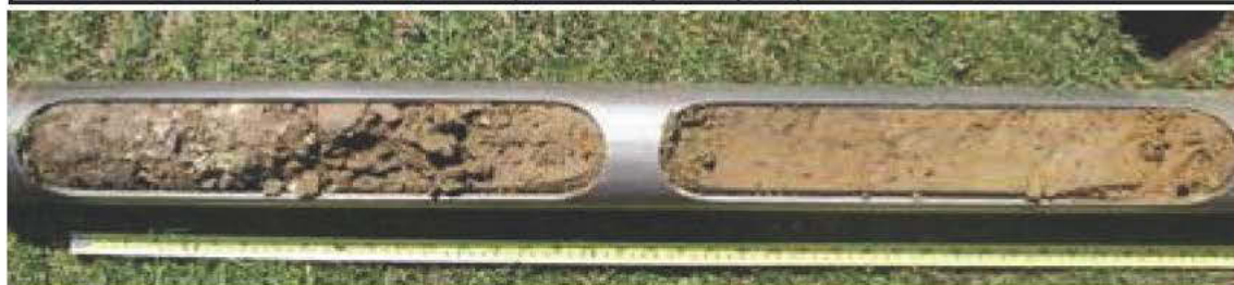
Figure 179 Core E. Base of the scarp. About 87 cm of the heavy clay overlying sand
