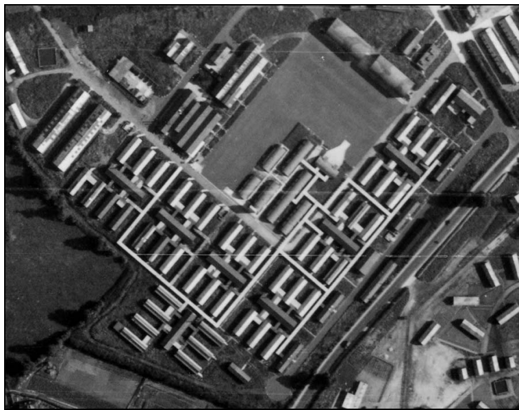
Figure 45 The completed hospital site (southern). Seven buildings were constructed on a parade ground and three of these are linked by the covered walkways that connect much of the site. The entrance building has two doorways and is highlighted in this photo by the lighter coloured tapering forecourt. Detail of RAF/106G/UK/1661 3164 12- Jul-1946 English Heritage RAF Photography
