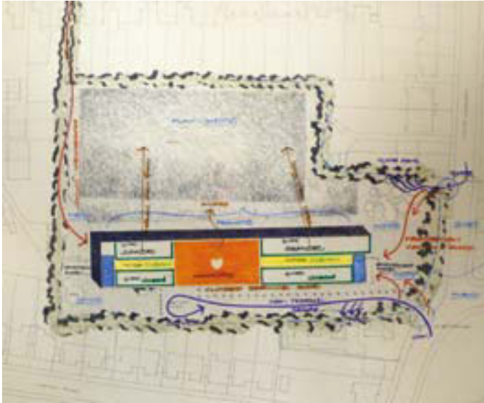
Figure 1.7: A 1966 design study by Team 4 (Su Brumwell, Wendy Cheeseman, Norman Foster and Richard Rogers) for the Homefield Preparatory School in Sutton. The drawing emphasises connections and contrasts: quiet/noisy; private/public; open/closed. The designation of 'entrance locks', service areas and dirty/clean processes is a reminder that the practice was then working on the Reliance Controls building in Swindon. Private practices often 'cross-fertilised' school design with their experience of other building types. Few public architects experienced such variety. (P5925001)
