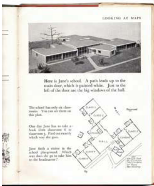
Figure 2.3: This 1958 textbook features a typical 'hen and chicks' plan. The school is Kingswood Junior School, Clay Hill Road, Basildon by Poulton and Freeman. From Jean and David Gadsby, Looking at Everyday things . London: A & C Black, p.69. Illustrations reproduced by permission of Essex County Council.
