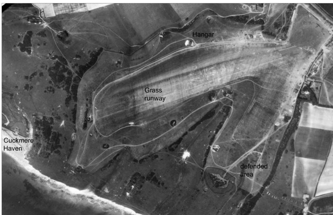
Figure 31 Friston Airfield – a Second World War emergency landing ground with a grass landing strip surrounded by perimeter roads, hangars and support buildings. US/7GR/LOC353 3025 29-MAY-1944 English Heritage USAAF Photography.
