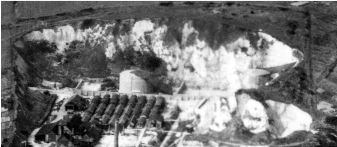
Figure 37 Fuel oil storage tanks in Meeching Quarry. The outline of the tanks when viewed from above was disrupted by the camouflaged netting, which was stretched down to the ground or up to the quarry's edge. RAF TQ4400/9 5-Sep-1943 English Heritage RAF Photography.
