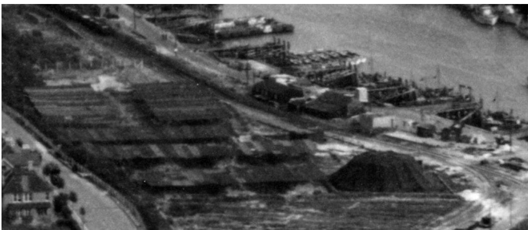
Figure 38 Camouflage netting concealing a storage tank (right) and a group storage buildings, possibly magazines near West Quay. RAF TQ4400/2 5-Sep-1943 English Heritage RAF Photography.
