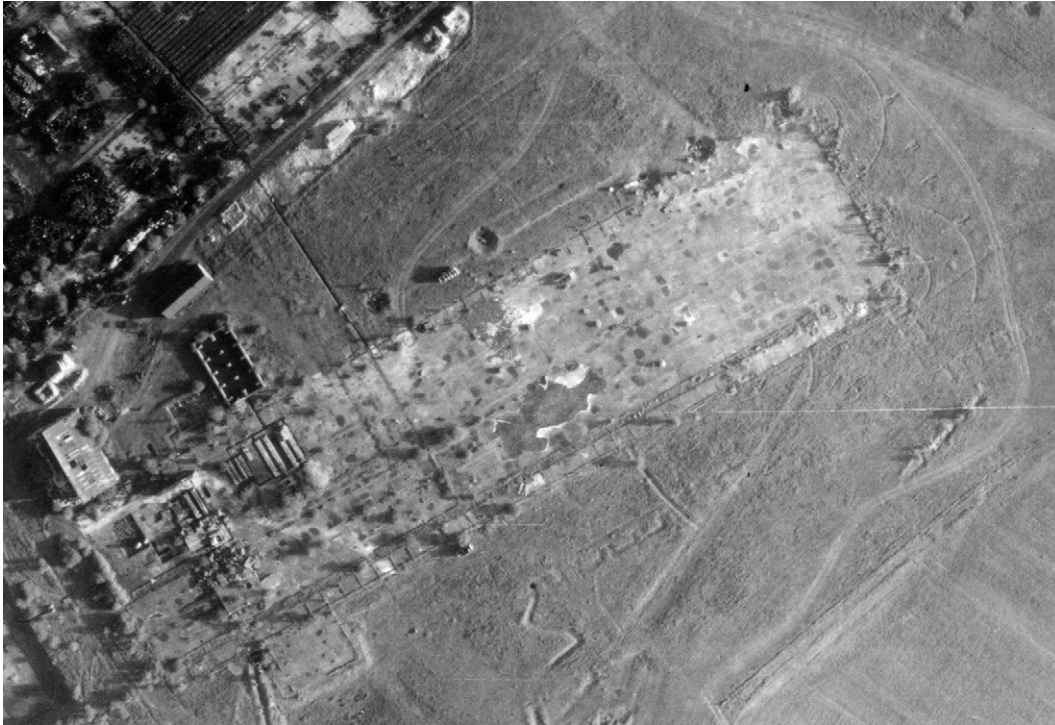
Figure 47 Outline of southern hangar at Kingsnorth taken in 1952. The arcs followed by the doors when opened or closed can be seen top right. Detail of RAF 58/856 3103 24-APR-1952 English Heritage RAF Photography.
