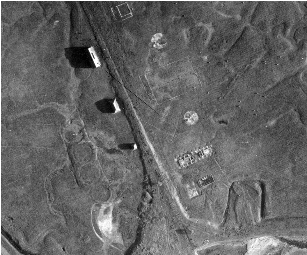
Figure 48 Remains of the hydrogen plant at RNAS Kingsnorth photographed in 1952. The faint outline of four circular gas holders can be seen on the left. Detail of RAF 58/4106 24-Apr-1952 English Heritage RAF Photography.
