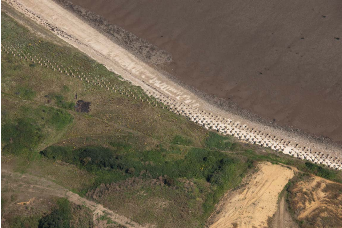
Figure 33 Coastal anti-invasion defences –dragon’s teeth on the beach on the Isle of Grain. Extract from 27197/011 19-Aug-2011 © English Heritage.
