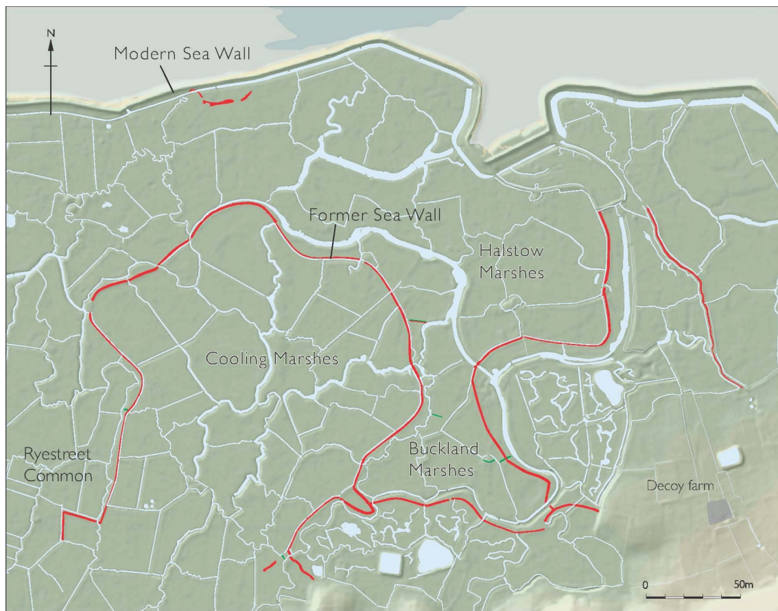
Figure 90 Map showing former seawalls identified from air photos and historic OS maps, not all of which survive. Unlike areas of Romney Marsh (see Eddison & Draper 1997), the pattern of walls on Hoo's marshlands does not show an overall steady advance of the reclaimed coast.
