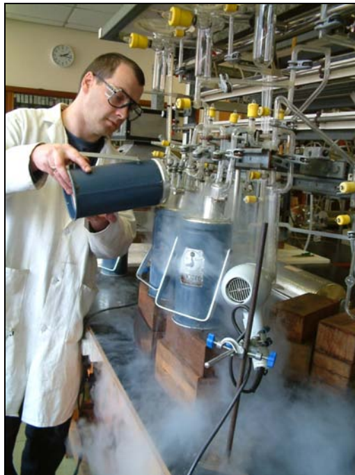
Figure 3: Sample combustion (photo Amanda Grieve)
