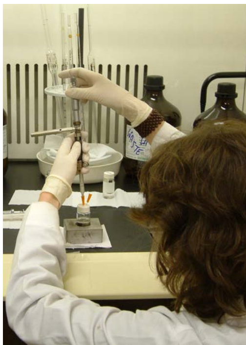
Figure 9: Preparing the benzene sample for counting (photo Amanda Grieve)
