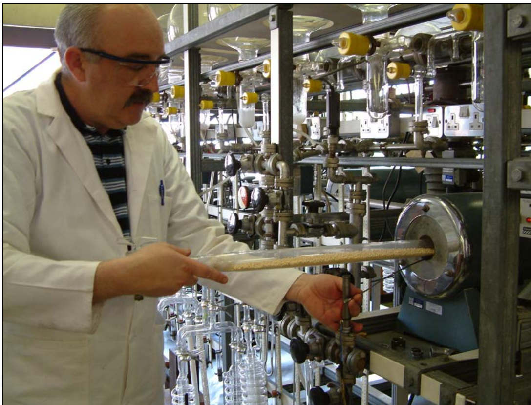
Figure 7: Loading the chromium oxide catalyst to convert the acetylene to benzene (photo Amanda Grieve)
