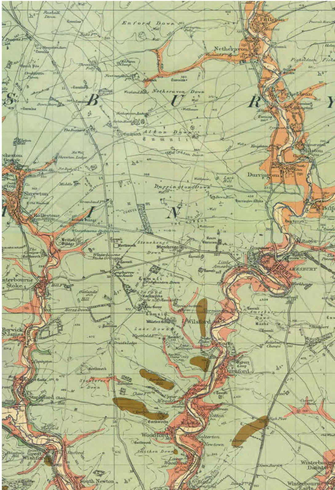
Fig 2.1 Geology around Stonehenge, combined from BGS sheets 282 (Devizes) and 298 (Salisbury). Green is Upper Chalk; note Clay-with-flints (brown) to the south; also Valley Gravel (orange) and Alluvium (yellow) in the river valleys. © British Geological Survey
