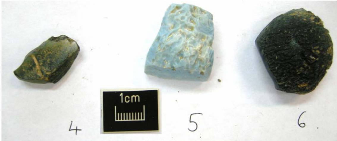
Figure 9: Typical greenish, better preserved appearance of HLLA glass (from Primrose Copse); the central example appears opaque because of phase separation, which is quite common in HLLA glass
