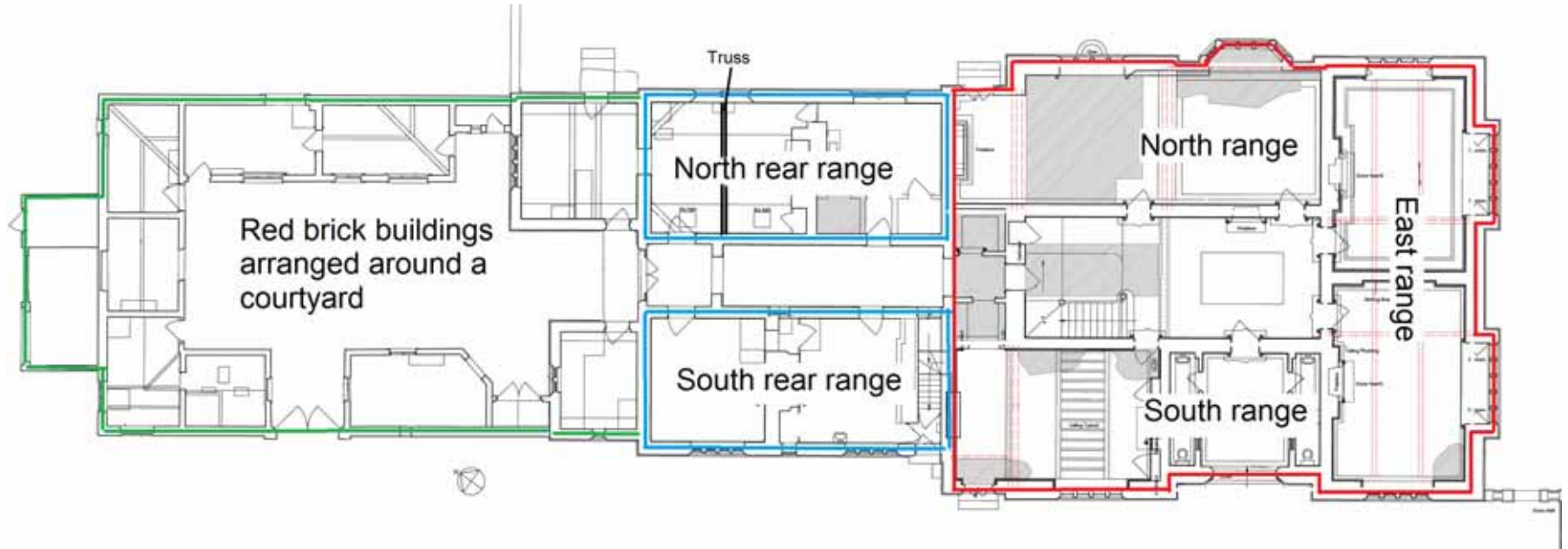
Figure 4: Plan of Sockburn Hall with areas investigated within the house outlined, and the location of the roof truss in the north-rear range marked (Blackett-Ord Conservation)
