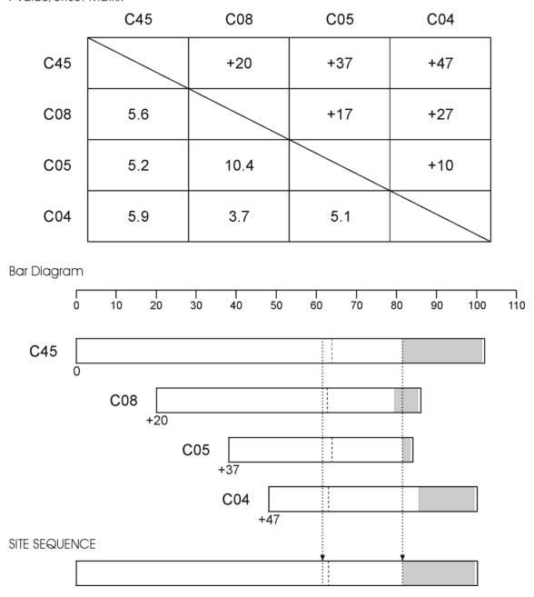
Figure A5: Cross-matching of four sequences from a Lincoln Cathedral roof and the formation of a site sequence from them
