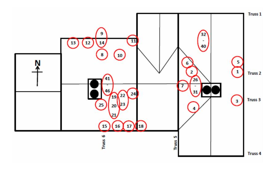
Figure 2: Simple schematic plan of Tonge Hall to show arrangement of the rooms and the general location of the sampled timbers
