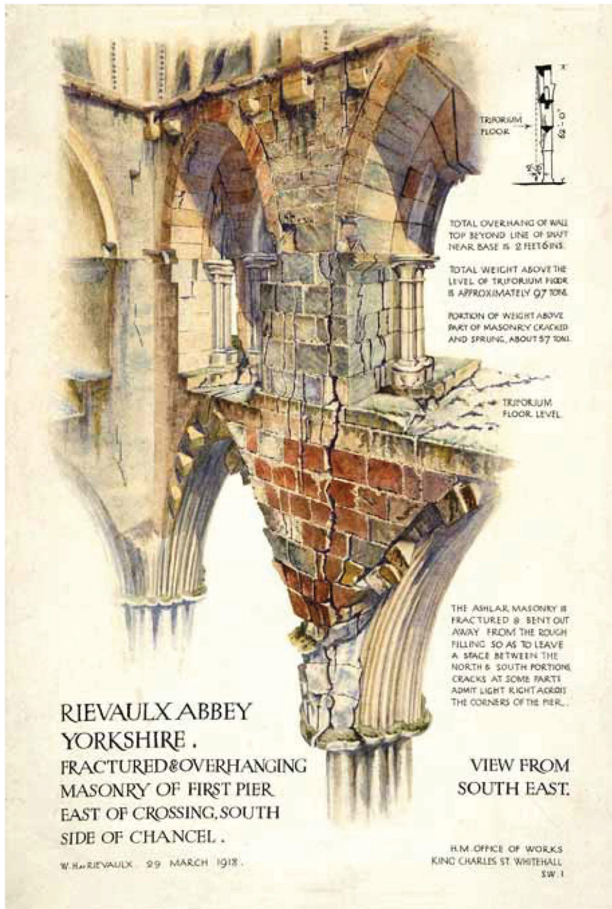
Figure 26: An Office of Works drawing showing the repair problems at Rievaulx Abbey in 1918. Copyright The National Archives. (File WORK 31/1609).
