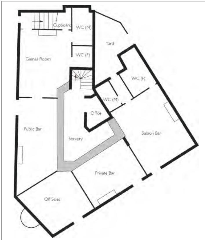
12.2.4 A reconstruction of the original ground-floor plan of the Army and Navy. (© Historic England, Phillip Sinton)
