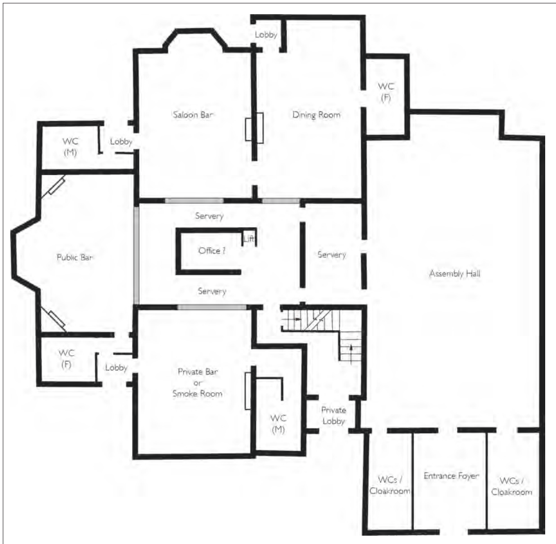
12.22.2 A reconstruction of the original ground-floor plan of the Green Man. The pub's layout has been much altered; this arrangement is based on the evidence of surviving features, on the plans of other comparable pubs of the time, and on the plan of the Green Man produced in 1995. (© Historic England, Philip Sinton)
