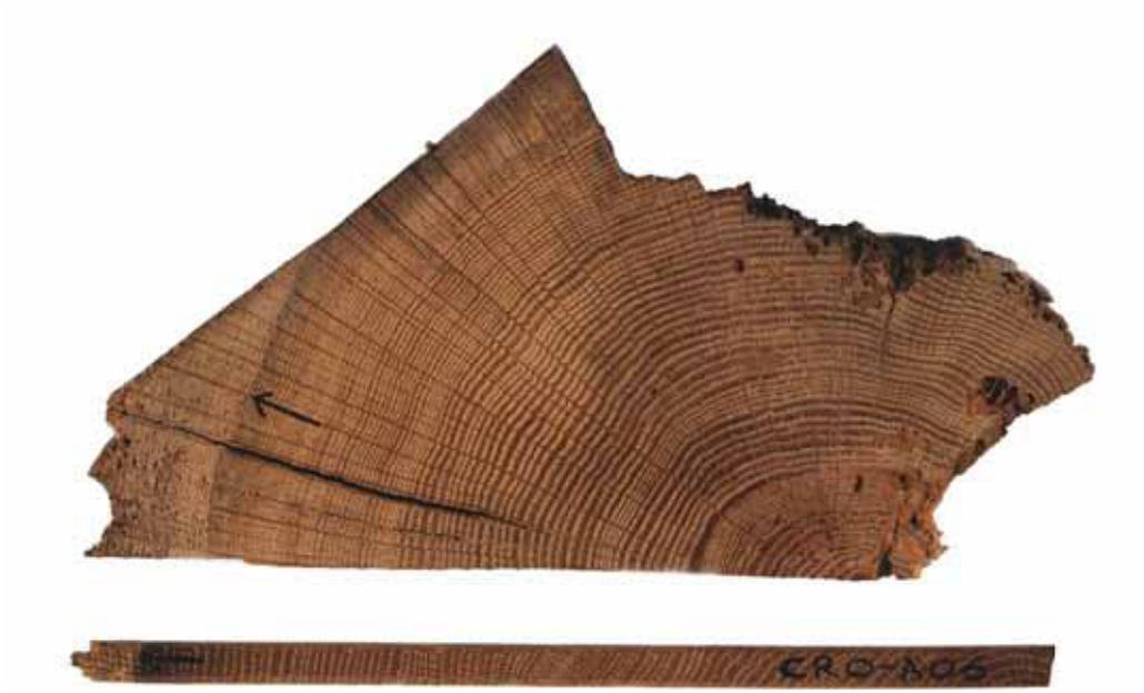
Figure A2: Cross-section of a rafter, showing sapwood rings in the left-hand corner, the arrow points to the heartwood/sapwood boundary (H/S); and a core with sapwood; again the arrow is pointing to the H/S. The core is about the size of a pencil
