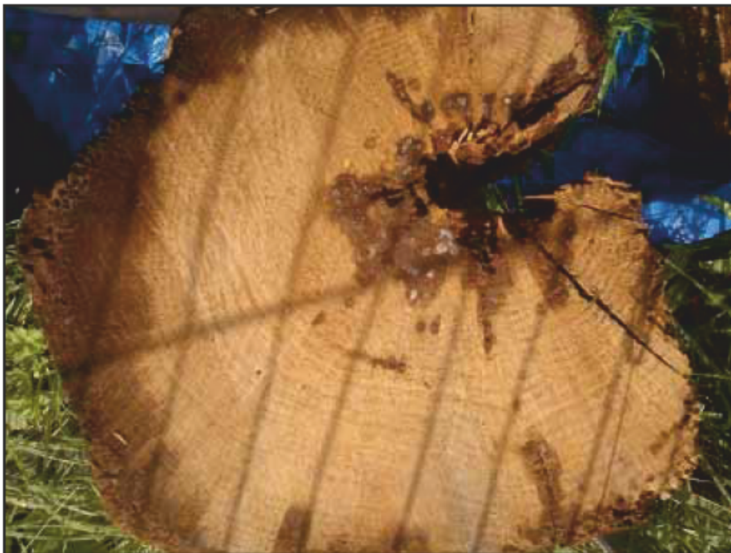
Figure 6: An ex situ spine beam from the Banqueting House ceiling; the wide growth pattern can clearly be seen (Robert Howard)
