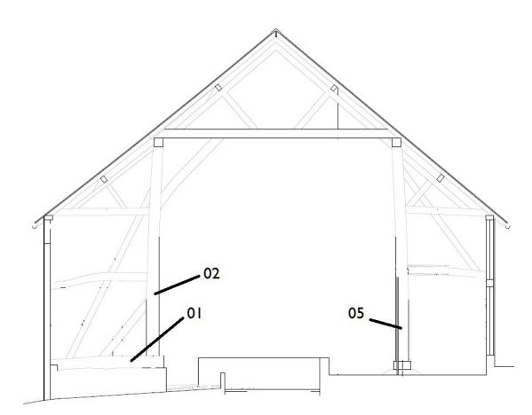
Figure 3: Drawing of truss B, showing typical truss form and the timbers sampled for dendrochronology. Adapted from an original drawing by Freeland Rees Roberts, Architects
