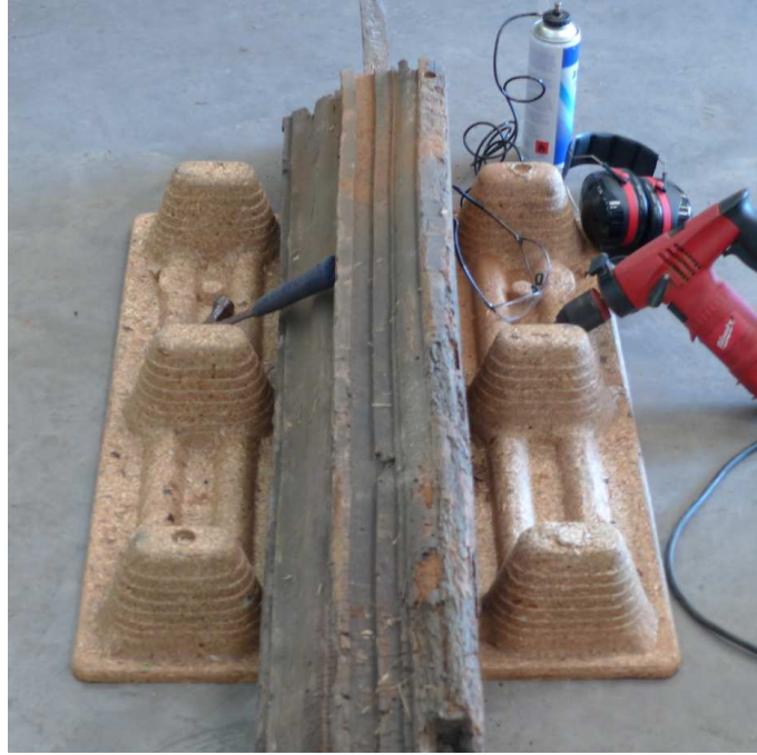
Figure 2: Jamb 88084596/3 from Brooke House, Hackney, during coring (Core 3), photo kindly supplied by Peter Marshall
