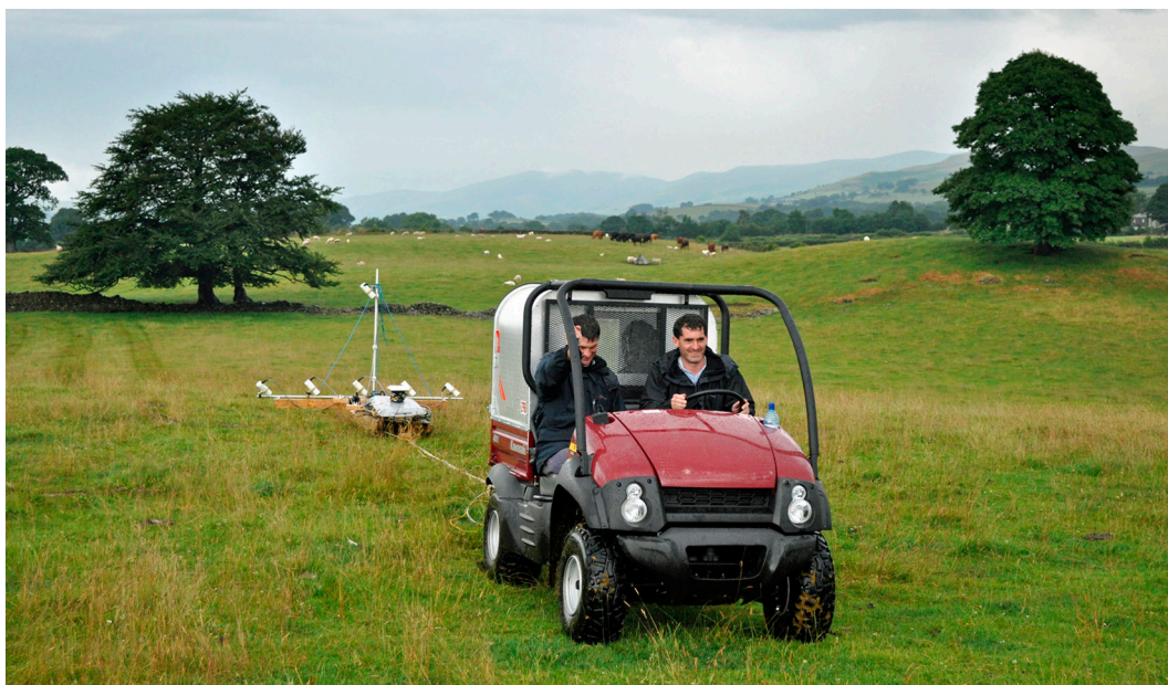
Fig 15: The caesium magnetometer towed array being used at Millbeck Farm. © Historic England, Pete Horne.
