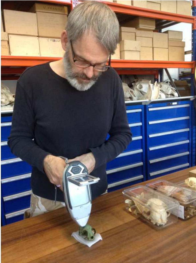
Figure 4 David Dungworth using portable XRF to test the elemental composition of the green pigment (photo: G Campbell)
