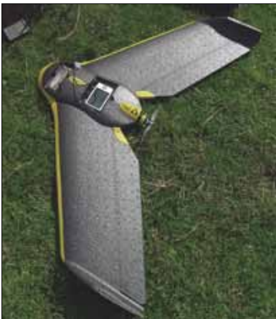
Figure 8: The autonomous Sensefly 'Ebee' small unmanned aircraft (SUA) used by UK Aerovision Ltd to capture the aerial imagery. Photo: David Went.
