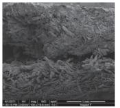
*Fig 25: Leather sample T 4, displaying a chaotic fibre structure.*
