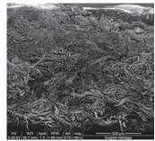
Fig 26: Leather sample NE 9 (no impregnation followed by non vacuum freeze drying), displaying a uniformly open fibre structure.
