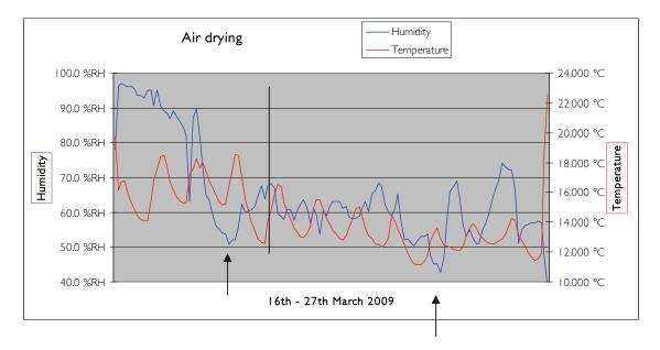
Fig 22: Temperature and humidity readings for the air drying method. The arrows indicate low points in RH where the sheeting was removed to weigh the leather. The vertical line marks 4 days after which the moisture loss seems to slow down.
