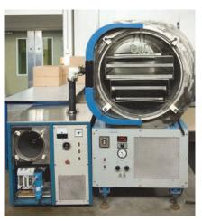
Fig 10: Vacuum freeze dryer.
