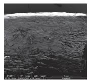
Fig 27: Leather sample NF 3 (no impregnation followed by air drying), displaying a compact fibre structure.
