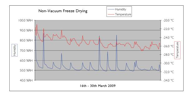
Fig 23: Temperature and humidity readings for the non-vacuum freeze drying method.
