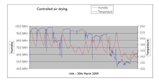
Fig 24: Temperature and humidity readings for the controlled air drying method.
