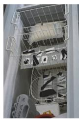
*Fig 9: Non-vacuum freeze drying in the chest freezer.*
