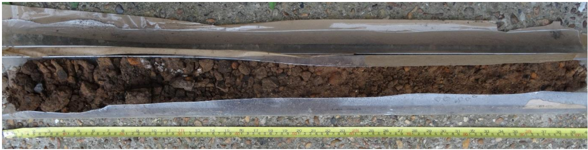
Figure 53. Borehole 5, 2.00 - 3.00 m (Most of this core is only partially in-situ).
