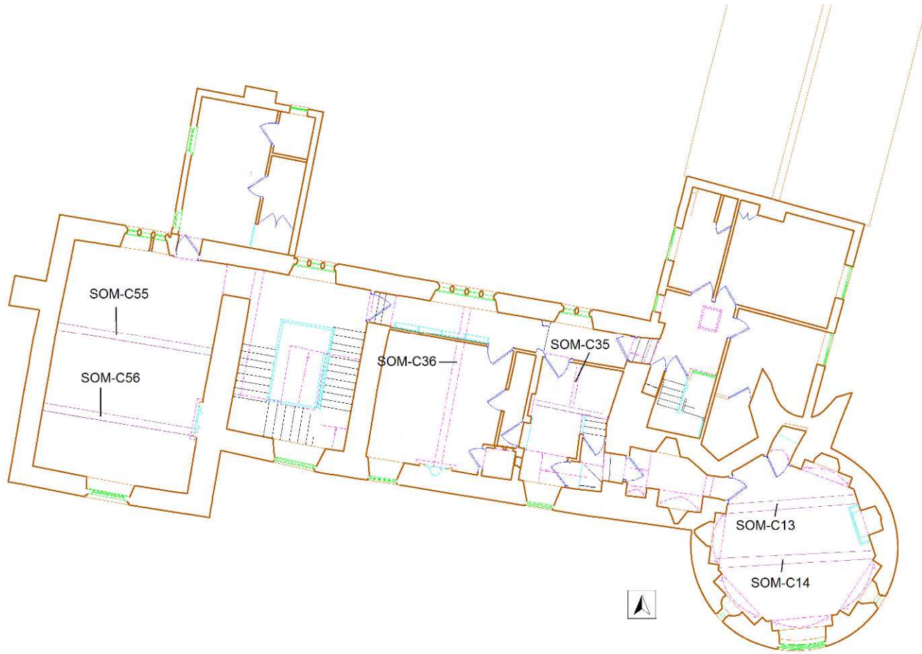
Figure 12: First-floor plan, showing the location of samples SOM-C13–14, SOM-C35–36, and SOM-C55–56 (after FAS Heritage)
