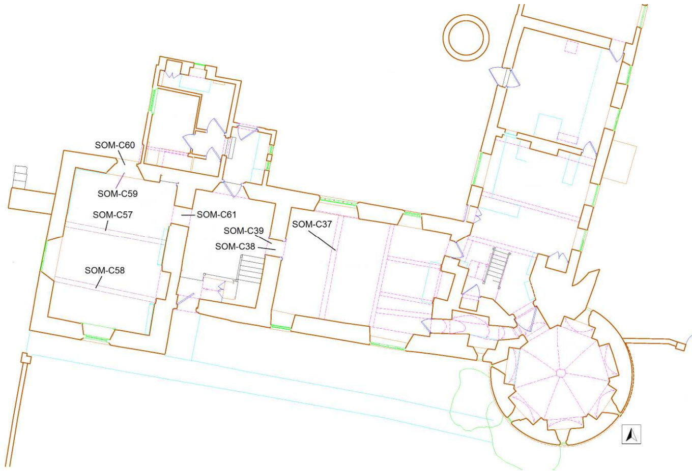
Figure 13: Ground-floor plan, showing the location of samples SOM-C37–39 and SOM-C57–61 (after FAS Heritage)
