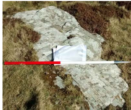
Figs 28 and 29: survey points 13 and 26 from the 1988 survey marked by iron pins in bedrock
