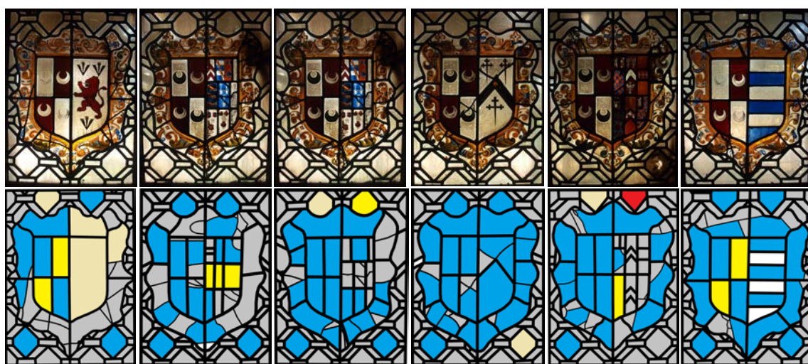
Figure 38. Wythenshawe Hall Window F8 (L1–L6) showing images of the windows and schematic colour-coded representations to indicate the type of glass (blue = HLLA; red = kelp; yellow = Leblanc soda ash; beige = mechanised; white = miscellaneous (flint glass); grey = not analysed)
